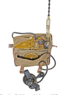
Russian R-352 special forces VHF FM radio used for activating and exploding the BON.
