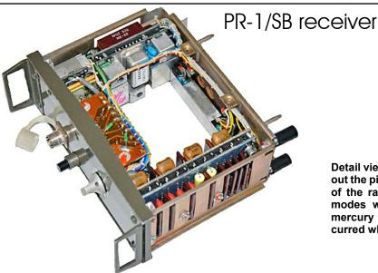
Internal view of a PR-1/SB receiver with top and bottom covers detached. An explosive charge with electric detonator fitted in the open space in centre. This detonator was connected to two black terminals located at the back of the chassis (on the picture bottom right).
