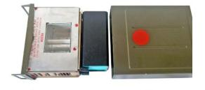
Top view of opened PR-1/SB showing the actual receiver (without explosive charge), rechargeable battery, cover and back cover screw.
