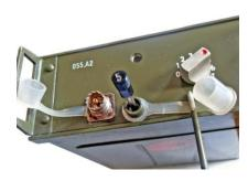
Detail view of aerial socket and time fuse pin. Pulling out the pin activated the booby trap and the time lock of the radio (if both were activated). When these modes were active and the receiver unlocked, a mercury tilt switch was activated. An explosion occurred when the device was tampered with.
