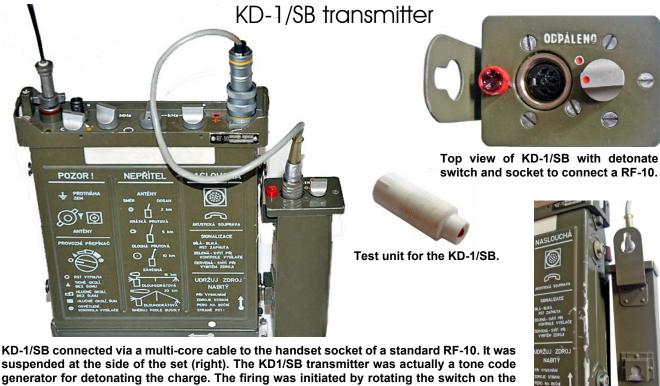
top of the transmitter to the 'Detonate' position. One of the three designated channels must be set on the RF-10 to match the specific receiver(s) of the SBON kit. In a kit were 4 receivers.
